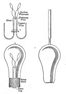
FIG. 152. Parts of a carbon filament incandescent lamp.
